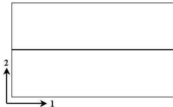
Figure 1: Blank for a violin top. The first direction indicates the axial direction (the direction of the fibre) and the second the radial direction.
